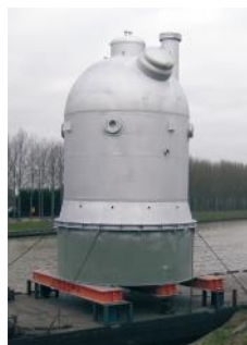
3rd stage separator
